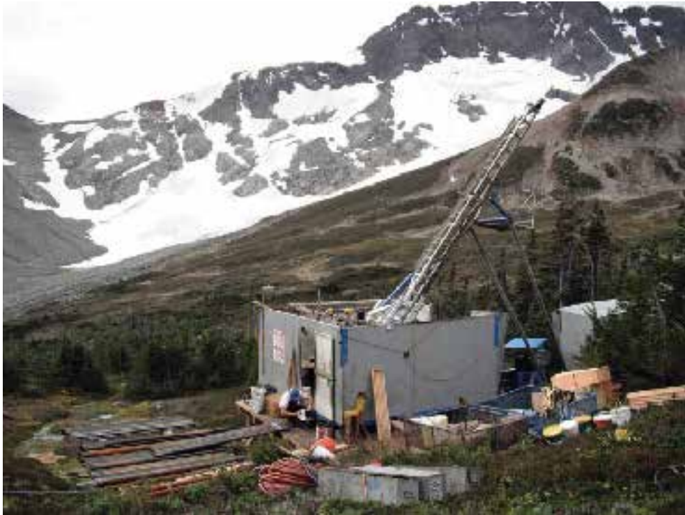
Figure 1: Diamond drilling rig on the Troitsa Property 2011
