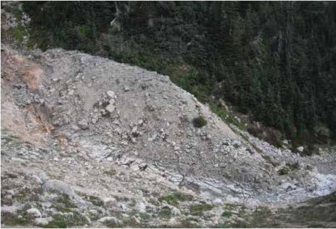
Figure 24: Photo from collar of Tr11-03, 04 towards Main Zone Photo is looking northeast down a steep slope towards bare rock in a ravine that is the site of the lower main zone channel sample. The rusty weathering zone on the left is bordered on its right side by a fault zone. To the right of the fault is a grey granitoid that is probably a dyke.
