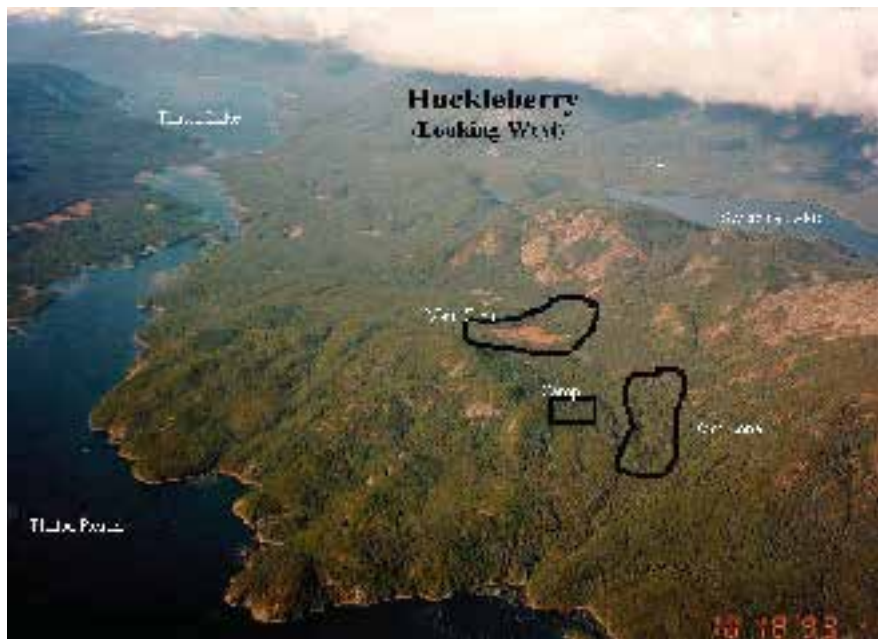
Figure 116: Huckleberry porphyry copper deposit Photo of the Huckleberry miner site prior to development in 1993 from the air looking west towards Taitsa Lake and the Coast Range mountains. The black outlined areas are the projections to surface of Cu mineralized zones lying within the pyrite halo outside of the Huckleberry stock. Photo from a presentation by Huckleberry Mines Ltd.
